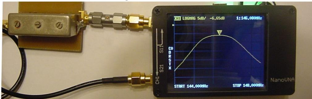
This picture shows that the filters Insertion Loss was 6.65 dB at 146 MHz's.
