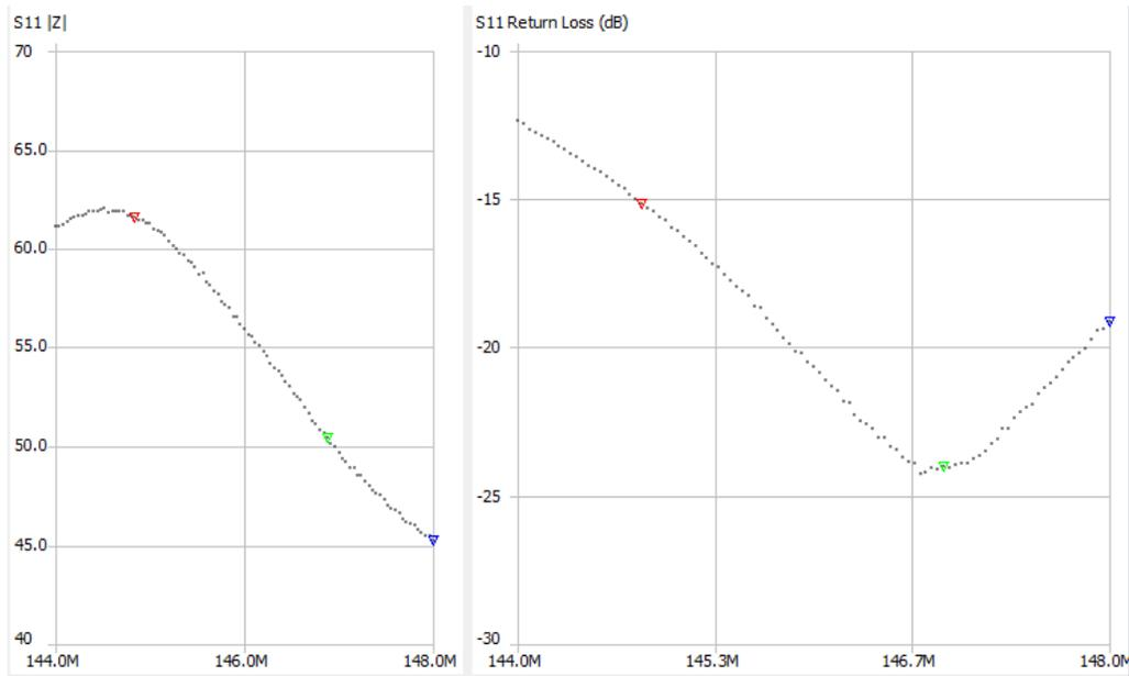
The start and stop frequencies include the complete 2M band. Looking at the Impedance (Z) chart, the impedance varied between 62 and 45 ohms. The **RED** marker shows the (Z) was 59.2 ohms. **GREEN** marker was 50.2 ohms and **BLUE** marker was 44.41 ohms. I set the **RED** marker on the Return Loss chart to -15 dB. Most antenna design engineers try to obtain RL of -15 dB because that equals to an SWR of about 1.5:1.
