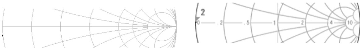
Both VNA's show that a short trace was on the 0-ohm circle, but the NanoVNA shows there is a small amount of capacitance. The same short was used when VNA's were calibrated, so this error was caused by circuitry.
