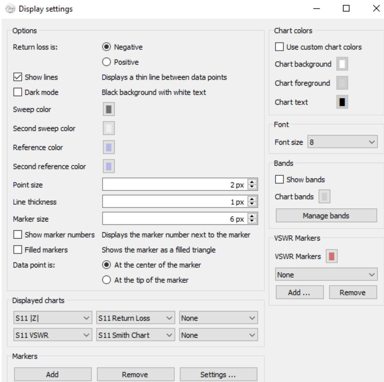
This screen allows you to choose how many display charts you desire and the type of measurement from the drop-down selection. In this case, I've chosen 4 charts and selected Impedance (Z), SWR, Return Loss and the Smith Chart. Note: I usually set the check the "Show Lines", change the "Sweep Color" to Black and "Second Sweep" to White.
