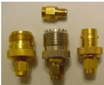
This VNA uses SMA connectors because this type of connector maintains a constant 50 ohms into the GHz frequency range. It also provides an excellent transition from the printed circuit board's planer surface to the coaxial connection.
