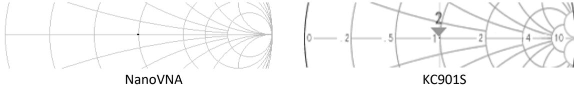
The NanoVNA and KC901S are terminated with 50-ohm loads that are pure resistance, no inductive or capacitive characteristics. Both VNA's show the trace point to be on horizontal resistive line and on the 50-ohm circle.
