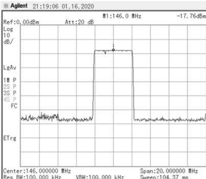
A receiver input impedance can be difficult to measure. Most VNA's output level is 0 dBm are more and could damage the receivers input stage. My MFJ-259B antenna analyzer output is 8 dBm. For repeater duplexers, the receiver's impedance must match the duplexer's 50 ohm impedance. I measured the NonoVNA's sweep output level at 146 MHz's and the level was -17.76 dBm. This is a safe level for any receiver, so the NanoVNA can be used to measure a receiver's input (Z).
